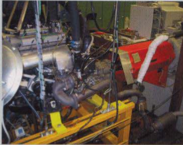
Turbocharged SI engine on a dynamic testbench
